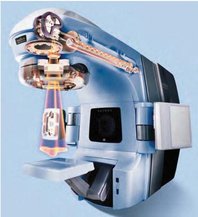
Figure 13.12 A shadow view of a C-arm linear accelerator. The electron beam (originating at upper right) is accelerated through a linear accelerator wave guide, selected for correct energy in a bending magnet, and then impinges on an x-ray production target. The x-ray beam (originating at target upper left) is flattened and collimated before leaving the treatment head. Also illustrated (downstream from the beam) is an electric portal imager that is used to measure (image) the beam exiting a patient. (From Varian Medical Systems, Palo Alto, CA, with permission.)
